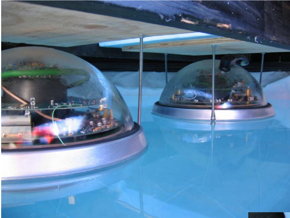
2 DOMs in liquid water in IceTop Tank
