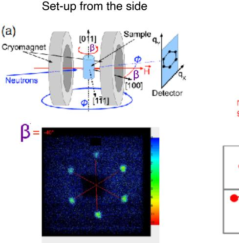
[011] х normal vector sample skyrmion lattice [100] Z [011] B ∥ ñ scattering pattern skyrmion lattice psd
