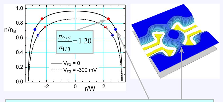
circling edge channel defined by density at saddle points in constrictions
