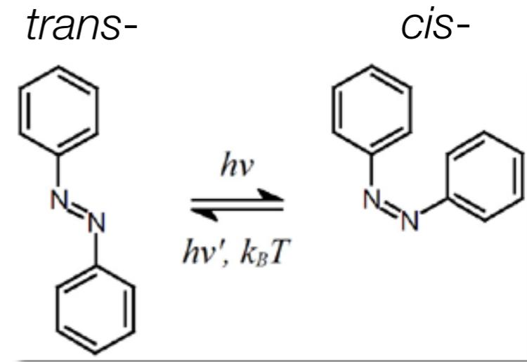
azobenzene photo-switches change isomerization with a frequency dependence in absorption
