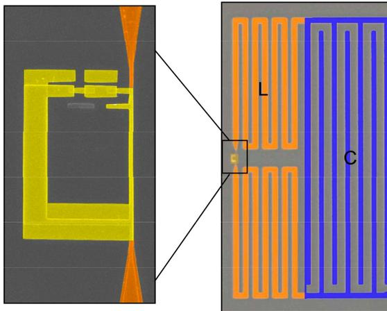
Flux qubit coupled to a microwave LC oscillator:
