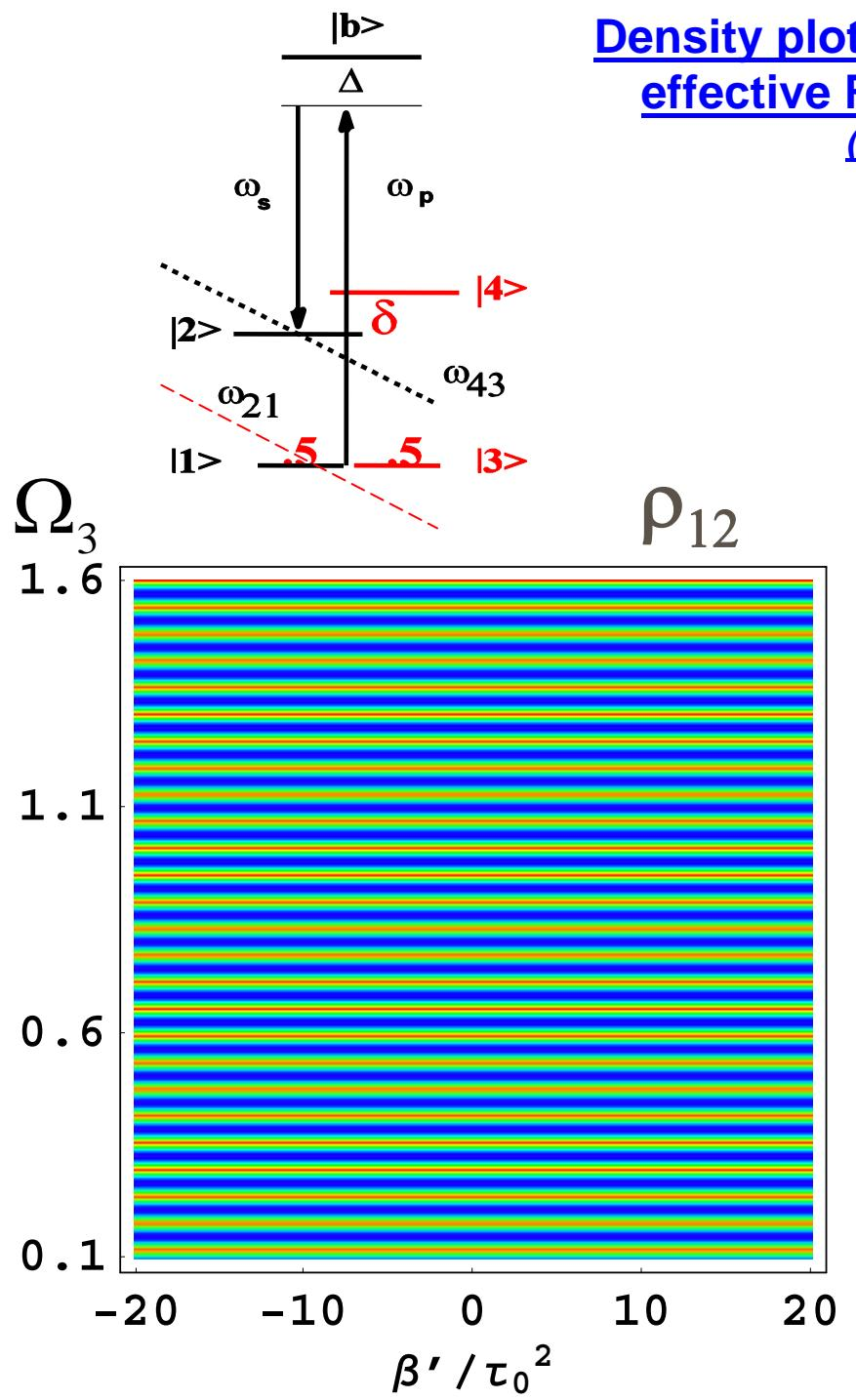
**Density plots of coherence as a function of the peak effective Rabi frequency and the spectral chirp, (the same for pump and Stokes pulse)**
