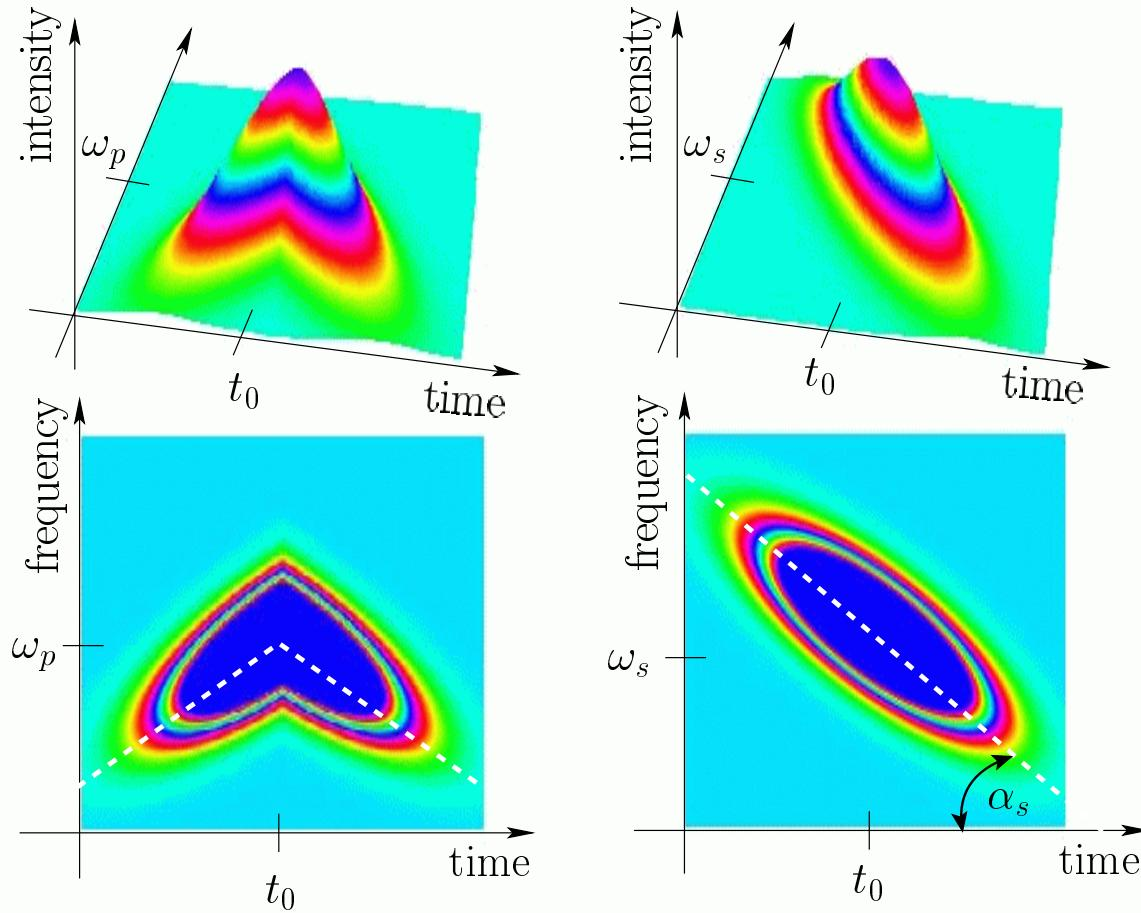
**The positive and negative slopes of white dashed lines on the density plots correspond to an upward and a downward frequency chirps.**
