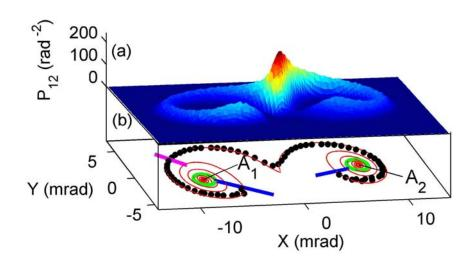
Switching trajectories in a parametrically excited micromechanical oscillator, Chan et al. (2008)
