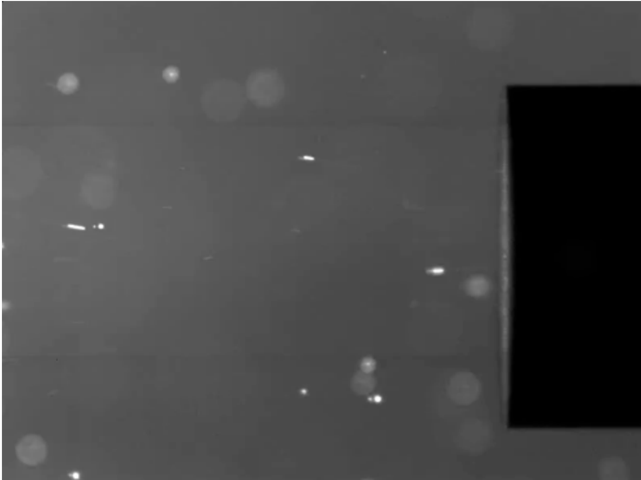
500µm glass beads hitting aluminum target
