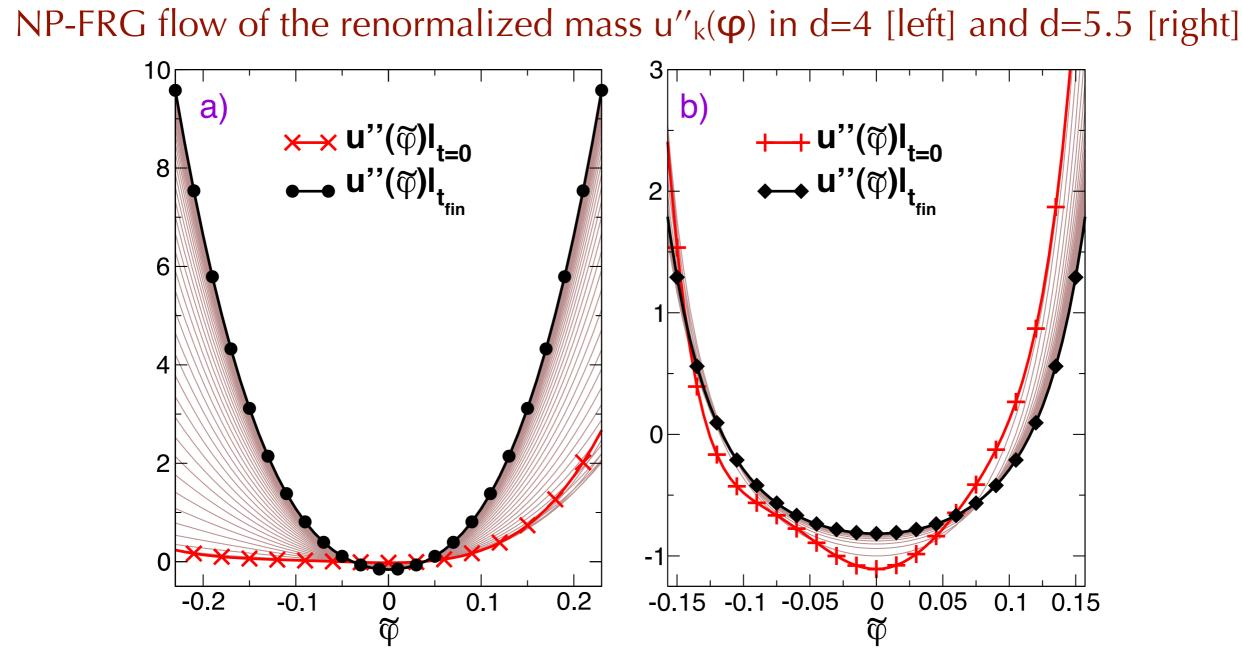
The initial condition is asymmetric (red) but it flows to a **symmetric fixed point** (black) that is **exactly the same one** obtained for the flow in the equilibrium case.
