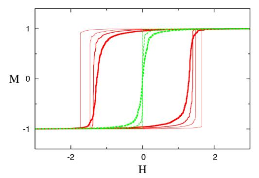
Dynamic versus static avalanches: Magnetization vs applied field at T=0 [Liu-Dahmen '06] Green: Equilibrium curves (ground state) Red: Ascending and descending branches of the hysteresis loop
