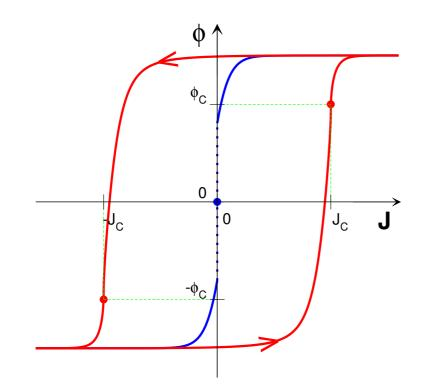
Magnetization vs applied field at T=0 at the value of the disorder  $\Delta_B$  for which the hysteresis curve has critical point(s).
