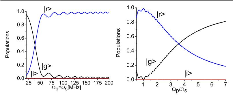
(left) Populations of the atomic states depending on the Rabi frequencies of the fields. Pulse duration 1µs, chirp rates 4.2 MHz/µs, one-photon detuning 1.5 GHz, two-photon detuning 1.5MHz; (right) Populations of the atomic states depending on the ratio of the pump and Stokes Rabi frequencies.
