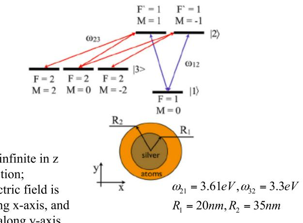
The wire is infinite in z direction; Incident electric field is polarized along x-axis, and propagates along y-axis
