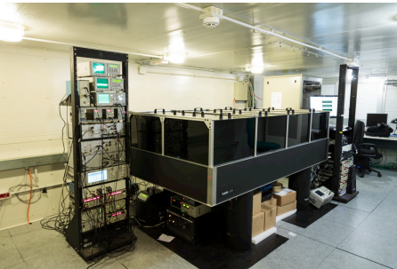
Astro-comb wavelength calibrator => RV ~1 cm/s
