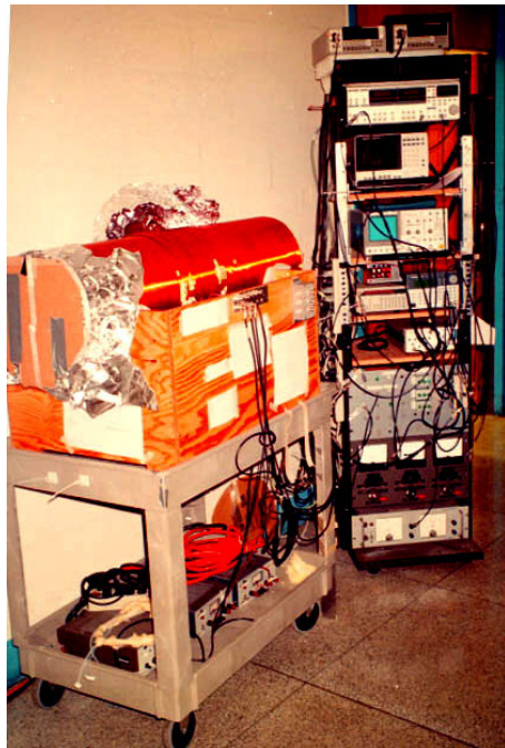
2.1 mT electromagnet MRI at CfA (repurposed noble gas maser)
