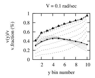
Shear can be induced without mechanically rough walls if side walls are not an obstacle, and driving wall is sufficiently frictional
