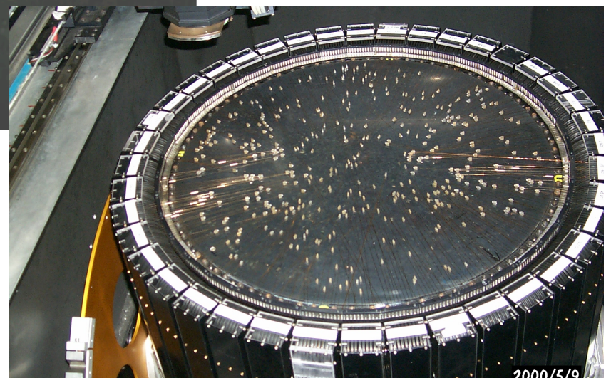
400 optical fibres positioned robotically
