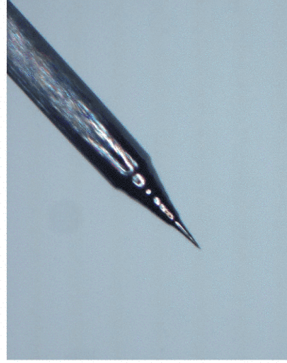
Electrochemically etched tungsten tip 200 nm tip radius
