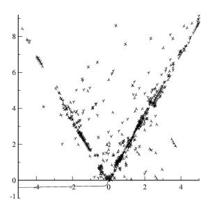
Many internal sources – no special dislocation nucleation from the crack tip.
