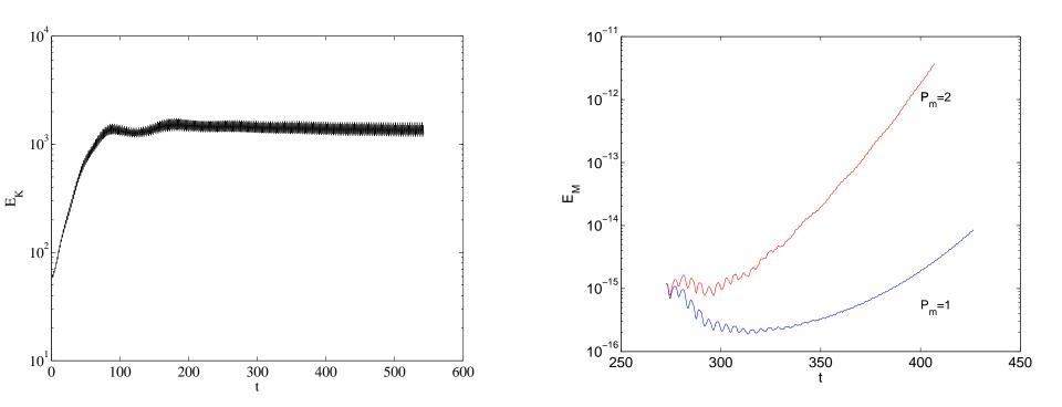
Small magnetic field is added at t=272. Right panel: Kinetic energy vs t Left panel: Plots of magnetic energy vs t for Prandtl number  $P_m = E/E_m = 1$ , and 2.
