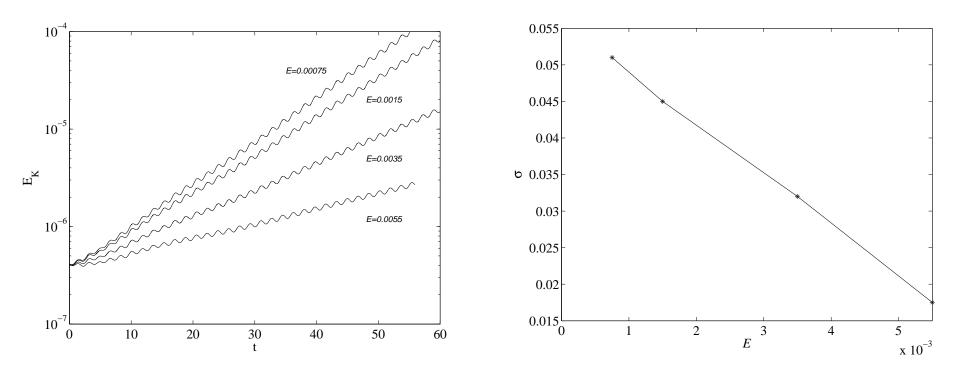
Kinetic energy vs t for calculations with several Ekman numbers for the case with c=0.8 and  $\Omega$ =0.25. (Inner grid: 513 points; outer shells: 71x71x61 points each.) Linear growth rate vs Ekman number for the case with c=0.8 and  $\Omega$ =0.25. Theoretical value of  $\sigma$  at *E*=0 is 0.054 (Kerswell, 1993).
