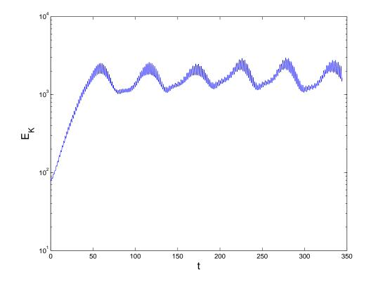
Kinetic energy vs t for the case with *E*=0.0011, c=0.8 and  $\Omega$ =0.25. (Inner grid: 51<sup>3</sup> points; outer shells: 83x83x61 points each.)
