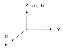
We consider the motion of a viscous fluid in a spheroidal container, which is rotating (rapidly) with angular velocity  $\omega_{\hat{z}}$  in a frame rotating (slowly) at angular velocity  $\Omega_{\hat{x}}$ . In this **precessing frame**,  $\mathbf{r} = \mathbf{x}\hat{x} + \mathbf{y}\hat{y} + \mathbf{z}\hat{z}$ ;  $\hat{x}\hat{y}\hat{z}$  are unit vectors.
