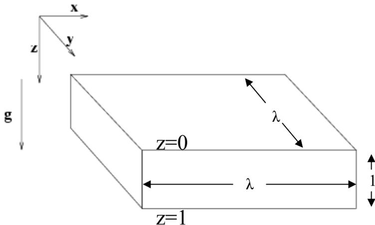
**Initially:** Fully-developed hydrodynamic convection. Density and temperature vary by an order of magnitude across the layer.
