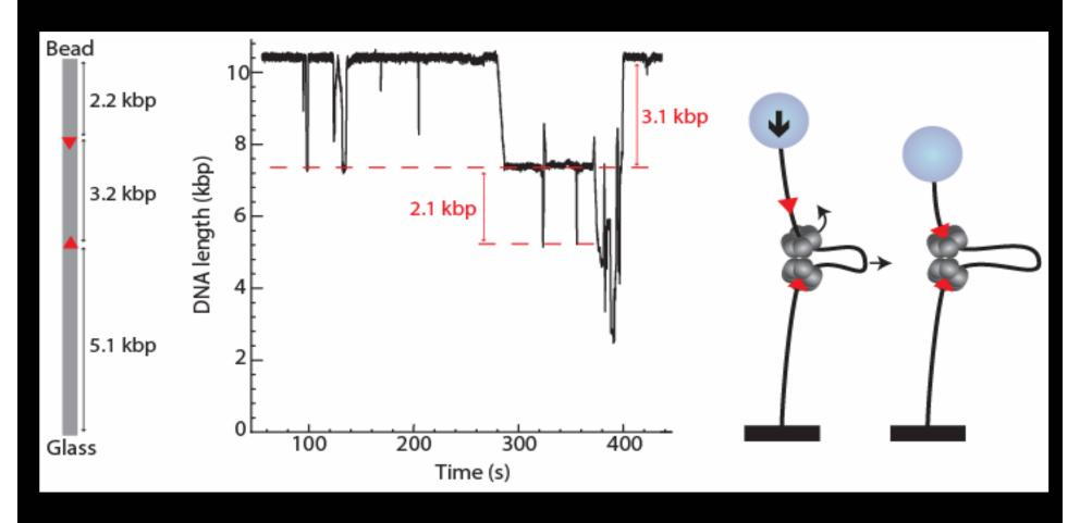
FtsK translocates from one KOPS, pauses upon hitting 2<sup>nd</sup> KOPS in anti-aligned direction
