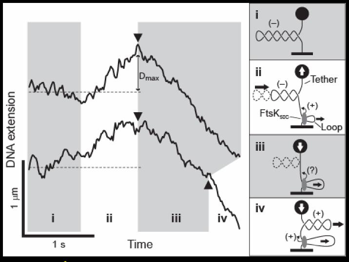
The 2<sup>nd</sup> buckling transition is inconsistent, unlike the 1<sup>st</sup> transition
