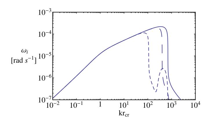
Growth rate vs scaled wavenumber for  $B=3\mu G$ ,  $n_i=1$  cm<sup>-3</sup>,  $n_{cr}v_D=10^4 {\rm cm}^{-2} {\rm s}^{-1}$ , and  $T=10^4 K$  (solid),  $T=10^6 K$  (long dashed),  $T=10^7 K$  (short dashed).
