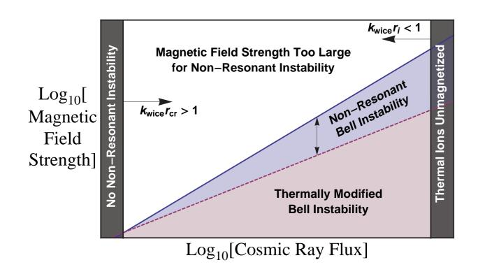
Schematic domains of nonresonant instability in the  $(n_{cr}v_D, B)$  plane, with  $n_i$ , T held fixed. The cosmic rays must be unmagnetized, the thermal ions magnetized.
