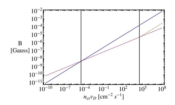
Instability domains for  $n_i=10^{-3}~{\rm cm}^{-3},~T=10^7 K$ . Above the blue line & outside the vertical bars only resonant instabilities exist. Between the red & blue lines the nonresonant instability is standard Bell, and below the red line, modified
